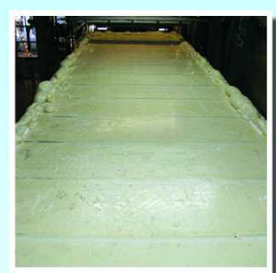
Foam in Place Roof to Side Continuous Seal
