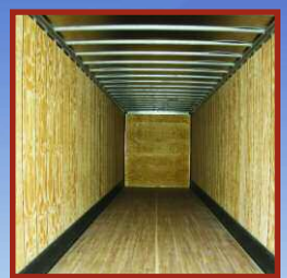
100.5" Plywood Lined Aluminum Roof Galvanized Roof Bows 24" Centers
