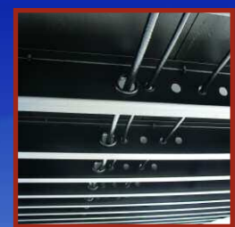
4" Wax Coated Cross Members with Integrated Electrical and Air Lines
