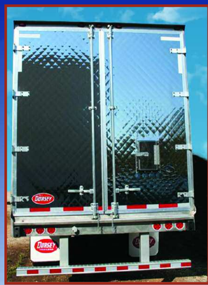
Stainless Rear Frame, Galvanized Door Locks, Stainless Quilted Rear Doors, LED Light Package Rear Header and Bumper
