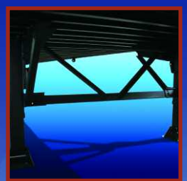
2-Speed Landing Gear, 50,000lb Capacity
