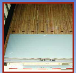
Threshold Plate Recessed at Front, Welded at Rear
