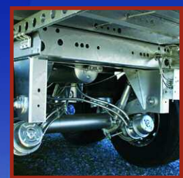
Suspension, Air-Ride Slider with Aluminum Color Resistant Paint
