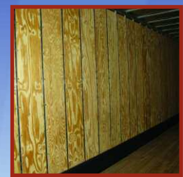
Plywood Lined 3/4" Logistics Posts
