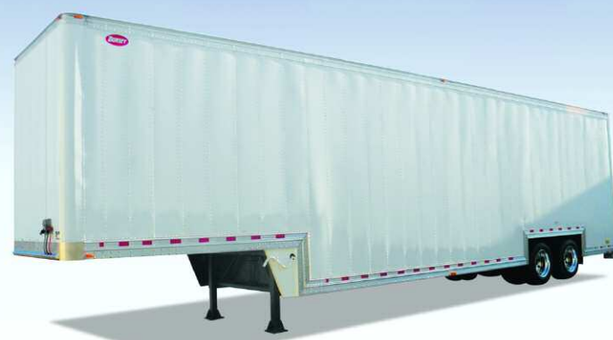
Stainless Rear Frame, Galvanized Door Locks, Stainless Quilted Rear Doors, LED Light Package Rear Header and Bumper
